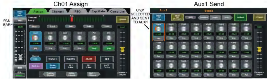
Figure 4.7a: No Linking, Ch01 sent to Aux1 only
