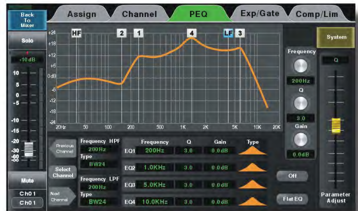
Figure 4.2: PEQ Parametric EQ Screen
