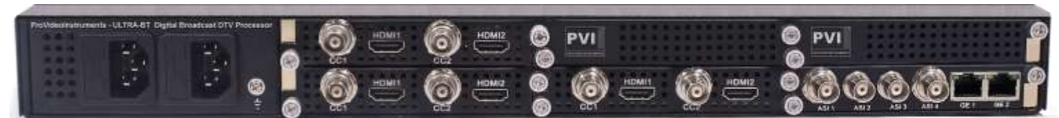
SKU: 0649070906012 ULTRA-BT-6HDMI-ADMUX - 6 HDMI In + 2 ASI In + 3 ASI Out + 2 IP In + 1 IP SPTS RJ+SFP Out + 1 IP MPTS RF-SFP Out - 2 Free Expansion Slots
