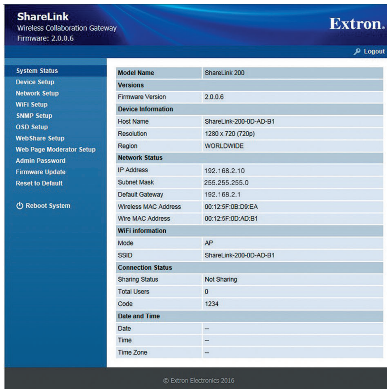
Figure 23: Use the gateway’s embedded Web pages to set up the ShareLink 250 Series unit, including updating device firmware.
