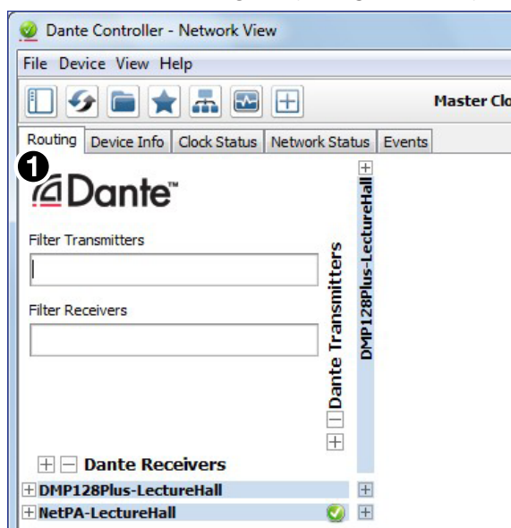
Figure 20. Dante Network View Screen, Routing Tab
