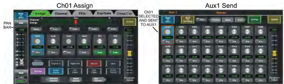
Figure 4.7a: No Linking, Ch01 sent to Aux1 only
