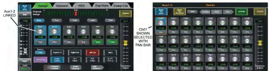
Figure 4.7c: Aux1-2 are linked, Ch01 sent to Aux1-2 and assigned to Main mix
