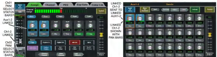
Figure 4.7d: Ch1-2 Linked, Aux1-2 also linked, both can be routed to Main mix
